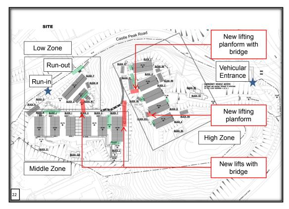
Site plan showing entrances (blue star), new ramps (green), new lifting platforms/lift towers and bridges (red)
