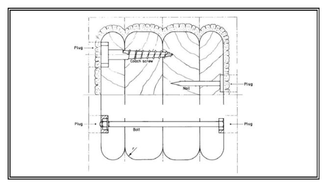
Figure 3 Charred timber section with steel connections to BS 5268 Part 4.1
