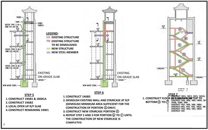
Sequence of rebuilding the exit staircase (ST-1) within the existing staircase tower
