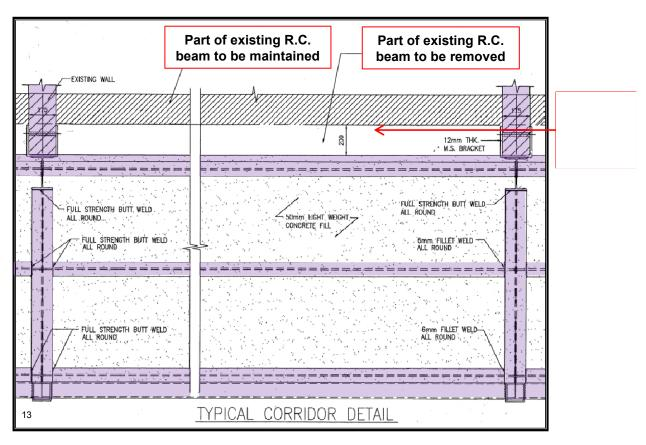
Details showing the new structural steel deck (in purple colour) fixed to the structural wall
