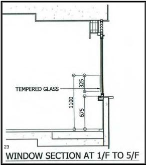
Tempered glass panel is installed above the existing parapet as protective barrier
