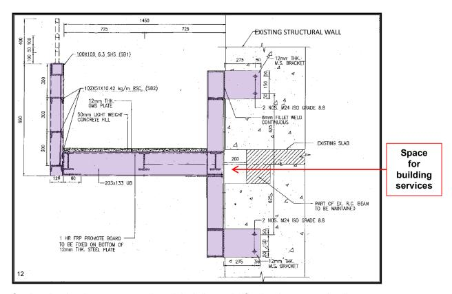
Section showing the new structural steel deck (in purple) fixed to the structural wall
