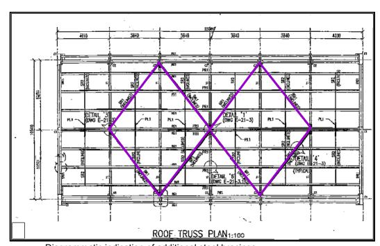
Diagrammatic indication of additional steel bracings
