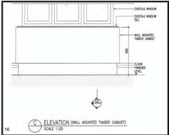
Section and elevation showing a cabinet installed in front of original window parapets
