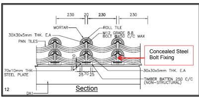
Fixing details of double-layer pan-and-roll tiles
