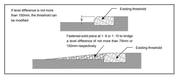
Figure 8 Installation of solid piece
