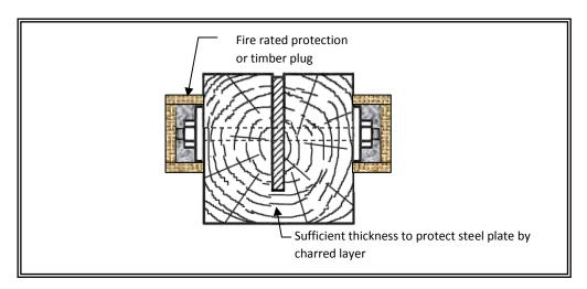
Figure 2 Steel strengthening plate in vertical sawn slot
