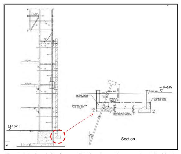
New steel structure, footing for accessible lift and ground improvement works by injecting cement grout into ground soil underneath existing footing
