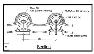
Fixing details of roof tile
