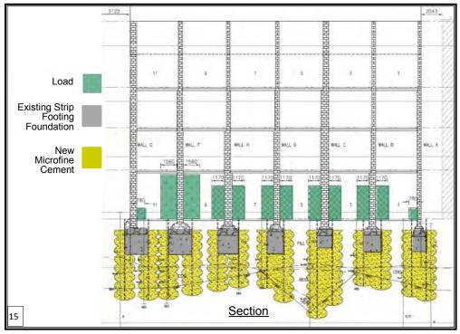
Strengthening of foundation by pressure grouting
