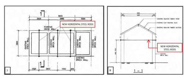
Plan and section showing strengthening works by horizontal steel rods in buildings at the Low Zone
