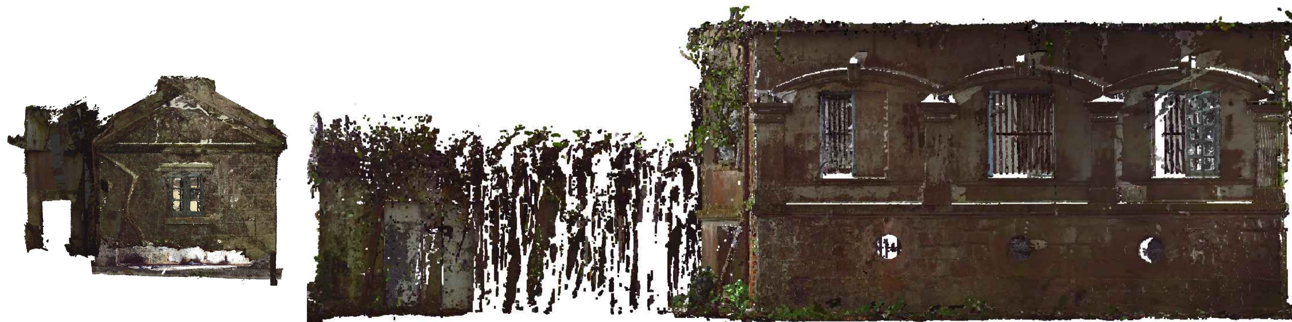
POINT CLOUD OF WEST ELEVATION
