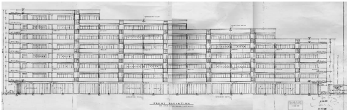
Fig. 53. The elevations of 13 Streets buildings reflecting the ascending height according to the flight landing skyline toward Kai Tak Airport.
